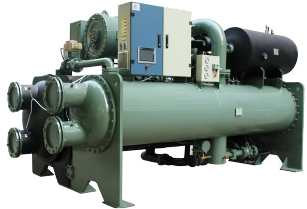
Centrifugal Water-Cooled Chiller, adopt two stage centrifugal compressor, equipped with self-developed high-efficiency falling film evaporator, COP up to 6.3 with R134a refrigerant. Suitable for larger industrial and
