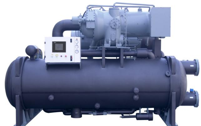
Centrifugal Water-Cooled Chiller, adopting special heat pump centrifugal compressor, equipped with self-developed high-efficiency falling film type evaporator, Cooling COP can reach 7.7 and Heating COP can reach 6.0 by using R134a refrigerant. Suitable for larger
